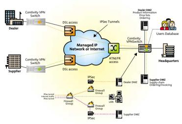
Figure 1: Nortel Networks Extranet IP-VPN Solution
